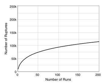
**Figure 33.** Number of above-water-level ruptures as a function of the number of simulated annealing runs averaged (for the reference branch). The maximum value on the y axis is the total number of possible ruptures ( $\sim$ 250,000).
