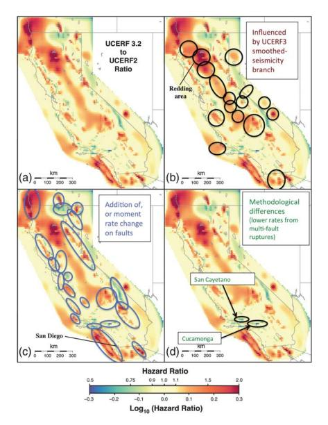
**Figure 31.** (a) Ratio of UCERF3 2%-in-50 year PGA map divided by that for UCERF2. The ground-motion prediction equations used for these calculations are the same ones used in the NSHMP 2008 maps. Ovals show areas where discrepancies can be explained by (b) addition of the *UCERF3 Smoothed Seism* option; (c) addition of new faults or average moment rate changes on existing faults; and (d) methodological changes in terms of including multifault ruptures.
