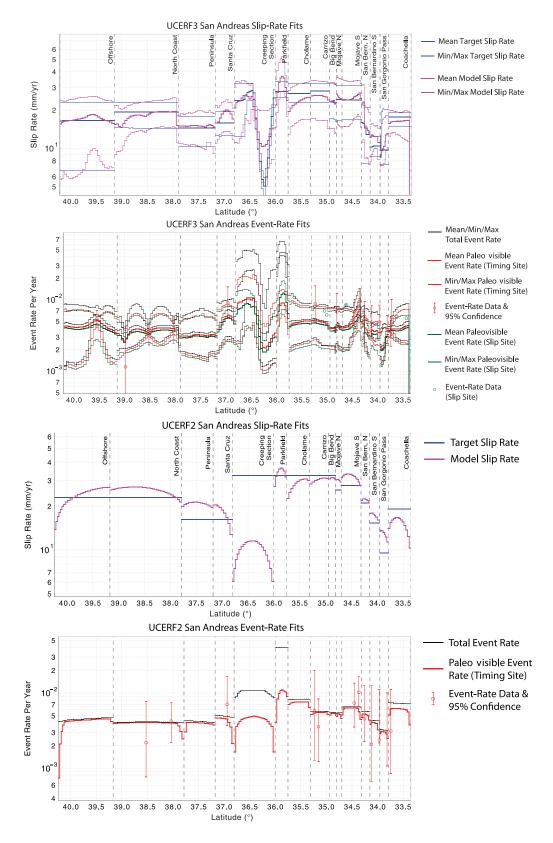
**Figure 20.** Latitudinal plots showing slip rate and paleoseismic data fits for the southern San Andreas fault, for both UCERF3 (top) and UCERF2 (bottom). The paleoseismic data on the UCERF2 plot are those used in that study, whereas the version of this figure in Appendix N (Page *et al.*, 2013) compares UCERF2 results to UCERF3 data. "Paleovisible" means that rupture rates have been reduced by  $P_r^{\text{paleo}}$  in equation set (2) (see Table 6) to reflect what might be seen in a trench.
