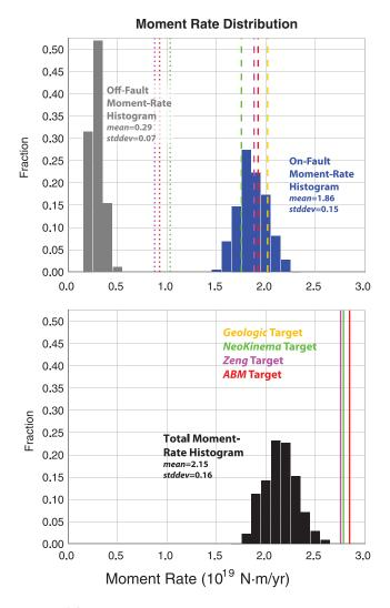
**Figure 24.** The distribution of regional moment rates implied by UCERF3 logic-tree branches (including their weights), in which blue represents total on-fault (including subseismogenic ruptures), gray is the off-fault, and black is the total combined rate. The vertical lines (dotted lines for off-fault and dashed lines for on-fault values) represent the various model targets as listed in Table 5 and as labeled in the bottom figure legend.
