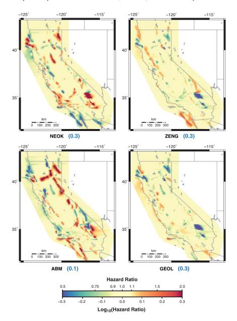
**Figure 32.** Branch-ratio maps showing the influence of each deformation model on 2%-in-50 year PGA. These ratios are obtained by averaging results over deformation-model subset branches and then dividing by the total average. Numbers in blue indicate the weights each model is given in UCERF3.
