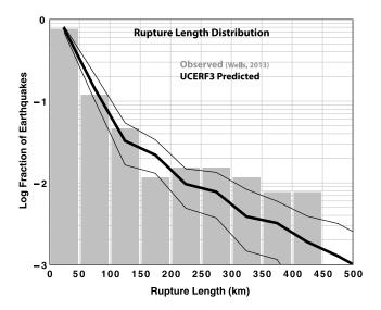
**Figure 21.** The observed rupture lengths from a global data compilation of 258 earthquakes (Wells, 2013), compared to the distribution implied by UCERF3 (thicker black line represents branch-averaged values, and thin lines represent the minimum and maximum among all branches). Curves have been normalized to density functions (values sum to 1) for comparison purposes.
