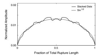
**Figure 13.** Mean rupture profile based on a stack of 13 mapped surface ruptures. The stack was obtained by normalizing the observed profiles to unit length and averaging them with their reflections about the midpoint. The details of this analysis are presented in UCERF2 Appendix E (Weldon *et al.*, 2007).
