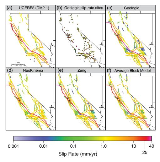
**Figure 7.** (a) Fault slip rates for the UCERF2 Deformation Model 2.1, (b) sites of geologic slip-rate constraints, and (c–f) fault slip rates for the four UCERF3 deformation models for *Fault Model 3.1*.
