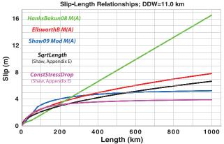
**Figure 12.** The magnitude–area (top) and slip–length (bottom) relationships used in UCERF3, which are documented in Appendix E (Shaw, 2013b). The M(A)-derived slip–length curves at the bottom assume an average seismogenic thickness of 11 km in converting area to length.
