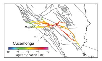
**Figure 22.** Map showing the rate at which the Cucamonga coruptures (participates) with other fault sections for the branch-averaged UCERF3 model (for *Fault Model 3.1*). Such plots for other fault sections are available in the Fault Section Participation Maps under U3 Supplementary Figures (see Data and Resources).
