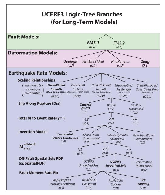
**Figure 3.** UCERF3 long-term model logic-tree branches with weights given in parentheses. The branches are organized by the basic model components in Figure 2: fault models (green), deformation models (purple), and earthquake rate models (blue). The branches and weighting decisions, as well as reference branch values for sensitivity tests (bold typeface), are described in the sections for each component. UCERF3 has a total of 1440 nonzero branches.
