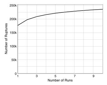
**Figure 35.** Number of above-water-level ruptures for branch-averaged solutions as a function of the number of simulated annealing runs on each branch (for *Fault Model 3.1*). The maximum value on the y axis is the total number of ruptures (~250,000).
