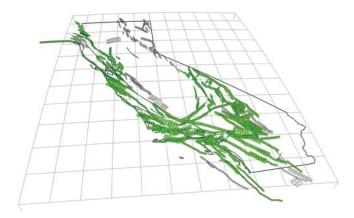
**Figure 11.** UCERF3 *Fault Model 3.1* sections divided into an integer number of equal length subsections (lengths equal to, or just less than, half the section's seismogenic thickness). All subsections shown in green are connected to all others in green without jumping more than 5 km between faults.
