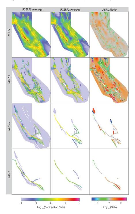
**Figure 28.** Branch-averaged participation rate maps for UCERF3 and UCERF2 and for the ratio of the two (UCERF3/UCERF2). For the ratios, zero values are white, values above the color scale maximum  $(10^3)$  are black, and infinite values are white (where the UCERF2 denominator is zero). These plots have had aftershocks removed in order to make the comparison to UCERF2. The zero patches in the UCERF3  $M \ge 7.7$  map represent the polygons for faults that have a maximum magnitude M < 7.7.
